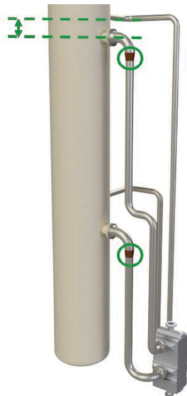
FIG. 6. Reboiler piping showing riser return expansion and column nozzle locations.
