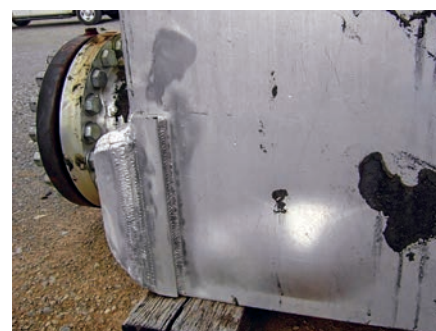
FIG. 12. BAHX damaged from water freezing internally.
