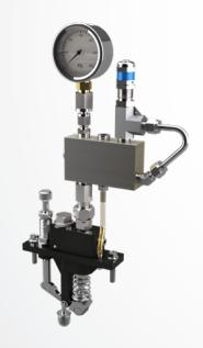
The lube guard pump assembly provides protection for the lubrication system by verifying that the camshaft is rotating while also indicating a low oil level condition in the lubrication box.
