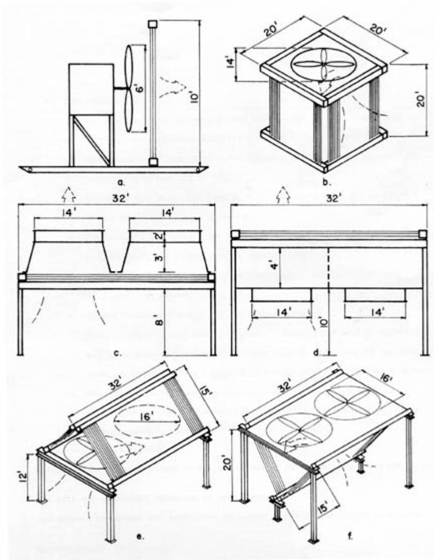
Figure 1 These figures illustrate various common types of dry air coolers.
