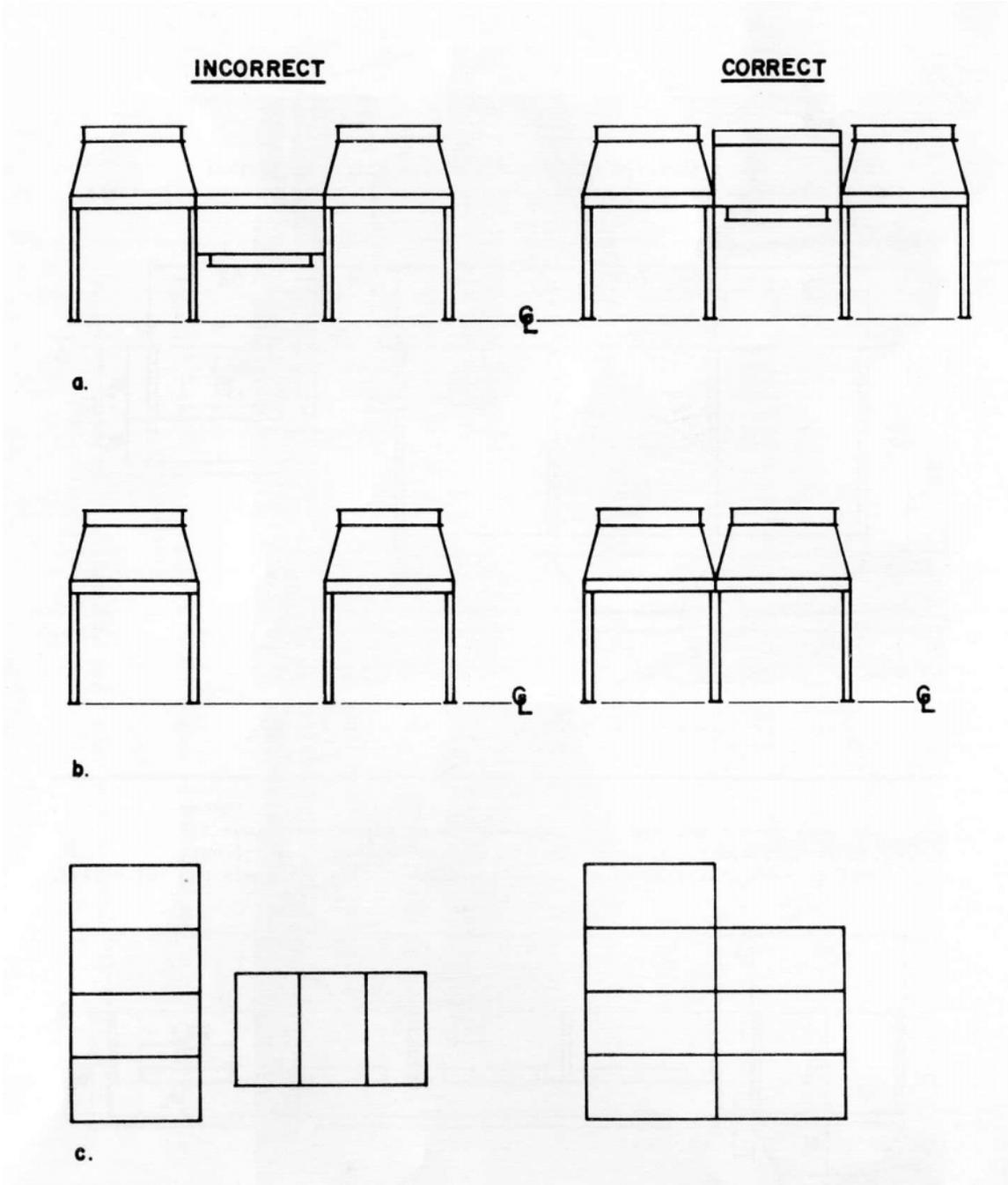
Figure 14(a)(b)(c) Incorrect and correct air cooler layouts.
