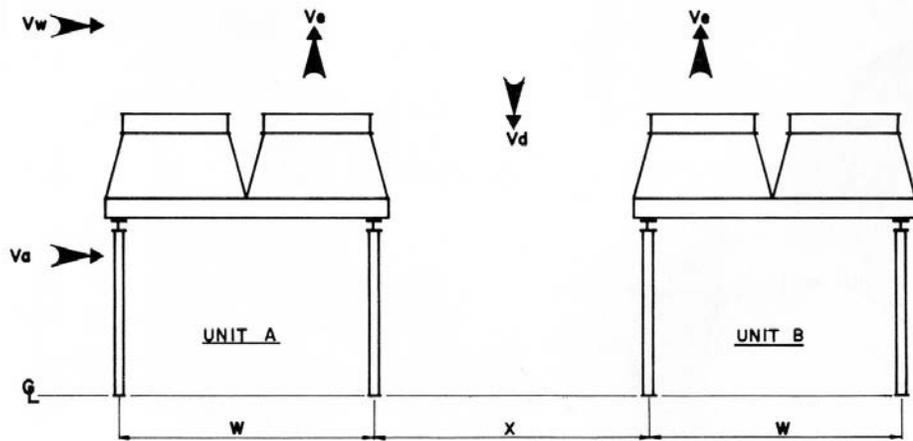
Figure 4 Force diagram and nomenclature for induced or forced draft air coolers.
