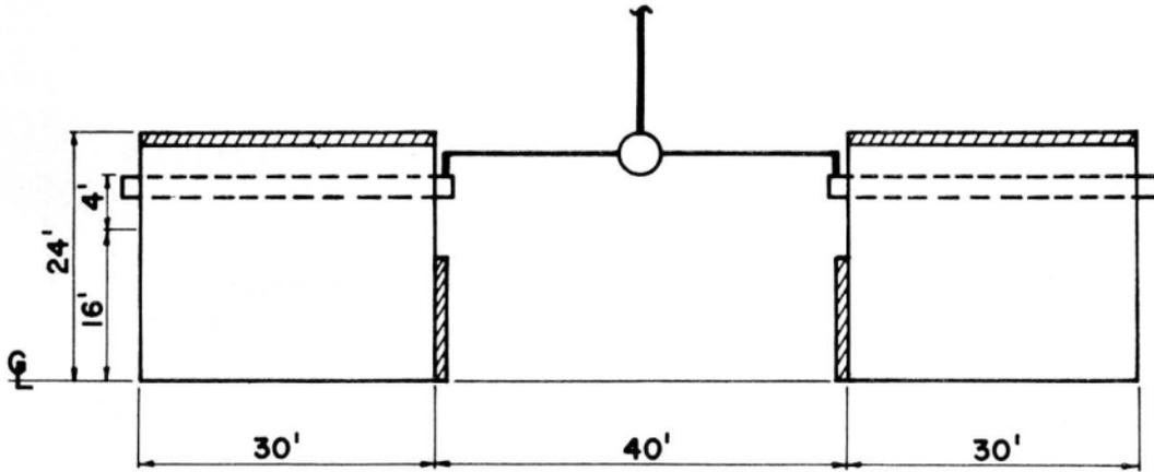
Figure 12 End elevation of two banks of forced draft air coolers installed in Alaskan plant. Hot air recirculated on both banks.
