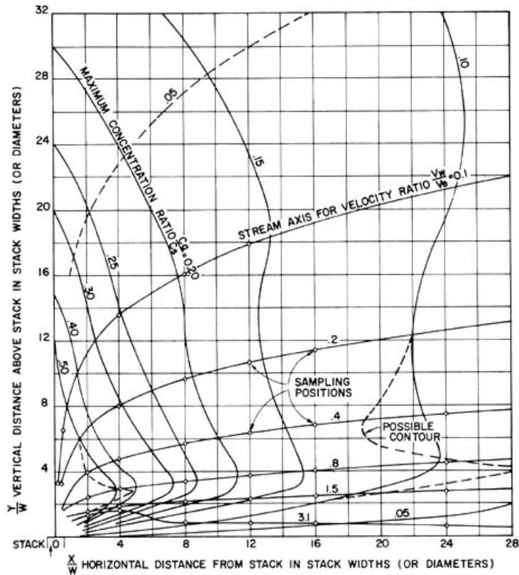
Figure 5 Maximum relative gas concentrations in undisturbed streams in the vicinity of a stack.
