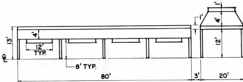
Figure 10 End elevation of air cooler layout in a southwestern natural gasoline plant. Hot air recirculation occurred where new induced draft air cooler was added to existing forced draft air cooler bank as shown.
