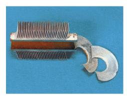
The WRAP-ON sample illustrates a serious corrosion condition between the fin and the tube, a situation that readily occurs in services because of loss of contact pressure at relatively low operation of temperatures with this type of fin. The helically wrapped and lapped type of fin has similar integrity problems.
