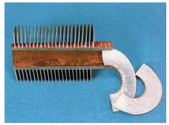
With the EMBEDDED sample, notice that there is a loss of tube wall due to depth of embedment groove, and that the products of corrosion are plainly in evidence for the length of the steel tube including to the base of the groove, under the fin. It is the presence of these corrosion products that results in loss of thermal capability.
