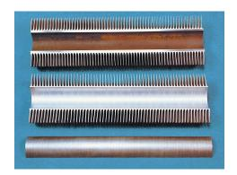
Note the EXTRUDED sample that the contact surface of both the aluminum and the steel are as bright and clean as when originally joined in a manufacturing process that absolutely ensures against oxidation and galvanic corrosion in the presence of water, air and air-borne impurities at the fin-to-tube interface, and which provides a residual contact pressure of 2000 psi.
