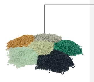
CPI 559 is a proprietary reinforced thermo-plastic material developed for use in CPI compressor valves
