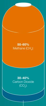
Traces of nitrogen (N<sub>2</sub>), oxygen (0<sub>2</sub>), water vapour (H<sub>2</sub>0) and other volatile organic compounds (VOCs) & hydrogen sulfide (H<sub>2</sub>S)
