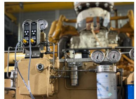
Lubrication system featuring the Proflo® EOS self adjusting lubrication pump
