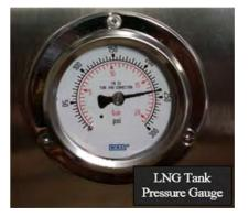
Note: If high tank pressures are present (above PRV set-point), determine primary cause of increased pressure and repair before returning truck to service.
