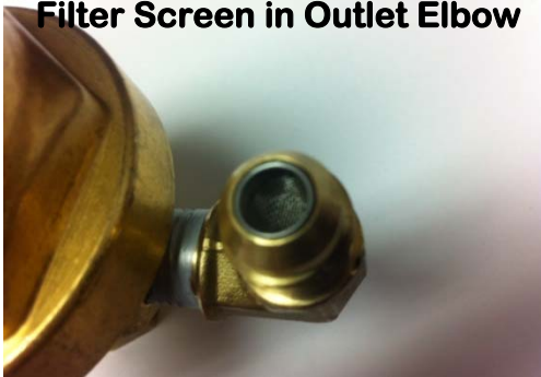
Filter Screen in Outlet Elbow
