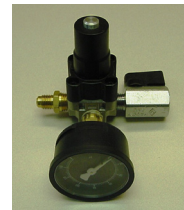
SMC Piston Style Regulators shown in color coded assemblies with gauges, and CO 2 ball valves. Gauges with stainless steel casings and color coded faces will be phased into use at a later date.
