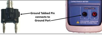
Capacitance Meter with Test Leads & separate BNC Test Lead Meter ports are polarity sensitive Capacitance Meter 11633137 Capacitance Test Lead 11385436
