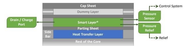
In practice, a user may install a BAHX equipped with Smart Layer<sup>™</sup> technology and, if they operate within the guidelines, will never see an indication of fatigue damage. In other instances, such as in severe service applications, the BAHX may operate normally for years before a fatigue indication occurs. When it does, the user is able to continue operating, but should plan to repair the unit within 3 months.
