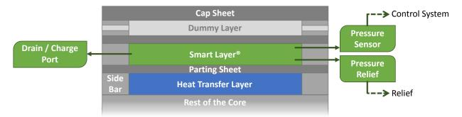
In practice, a user may install a BAHX equipped with Smart Layer<sup>™</sup> technology and, if they operate within the guidelines, will never see an indication of fatigue damage. In other instances, such as in severe service applications, the BAHX may operate normally for years before a fatigue indication occurs. When it does, the user is able to continue operating, but should plan to repair the unit within 3 months.
