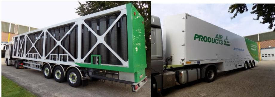
Today's state of the art solution for high pressure Hydrogen trailers is hitting the road in Europe. The unique design is due to European regulations covering trailers of this size. The 'inside the box' photo (*above left*) shows a system comprised of 135 interconnected, vertical, high pressure cylinders engineered and built by Chart's GOFA facility in Germany,
