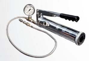
The CPI purge gun provides a convenient, cost effective method to remove air from the divider block system to ensure all lubrication points will receive lubrication immediately on start-up of the compressor.
