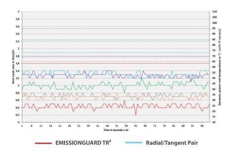
A selection of packing ring styles including other low emission rings from the industry were tested on CPI's test compressor. The vent leakage and piston rod temperature results are presented above.
