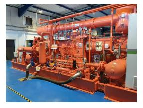
Tests have been conducted on CPI's Reciprocating Test Compressor, located in CPI's R&D laboratory, Feignies, France, which can operate up to 60 bar (870 psi) with either air or nitrogen, having a linear speed from 2.47 to 4.40 m/s (8.1 to  $14.4 \, \text{ft/s}$ ) and a rod diameter of 50 mm (~2").
