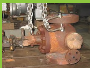
Images show Turbine Control Valve as received from customer and after overhaul
