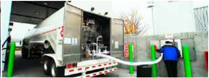
LNG Pressure Transfer Trailer making delivery
