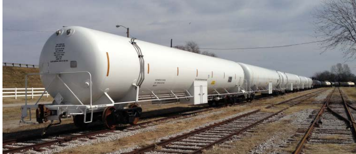
DOT-113C120W Tank Car. ~30,000 gallons net volume
