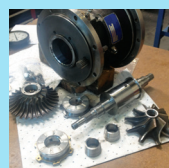
Customer-supplied Turboexpander-Compressor for evaluation and repair.
