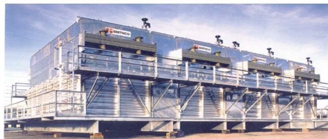
▲ Figure 4. A winterized forced-draft unit is outfitted with methods to control the process fluid temperature leaving the ACHE.
