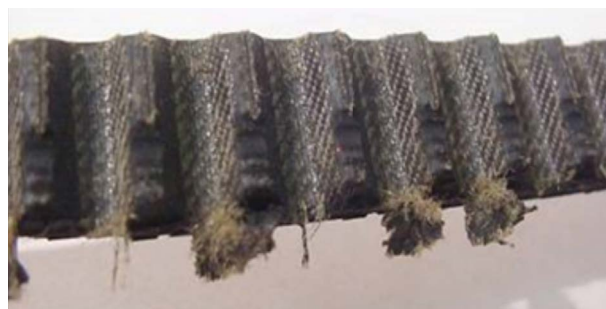
Examples of Pulley Misalignment
