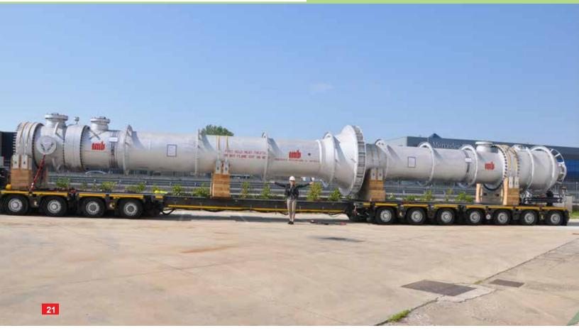
21 TEXAS TOWER, Vertical TEMA CES type HEx. for a Catalytic Reforming Unit, Gr.22 Cl.3 low-alloy steel - 19 meters long Tp.321 stainless steel tubes
