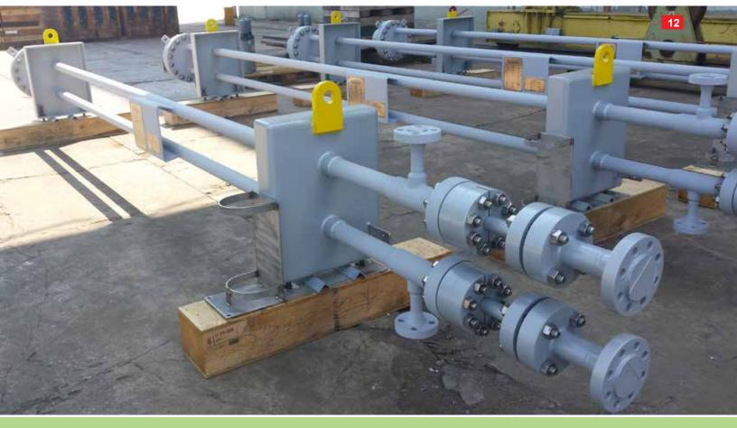
12 Double Pipe Heat Exchanger
