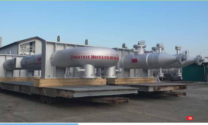
HAIRPIN HEAT EXCHANGERS -AN EFFICIENT ALTERNATIVE TO CONVENTIONAL SHELL & TUBE HEAT EXCHANGERS 10 Non removable bundle - HAIRPIN all welded
