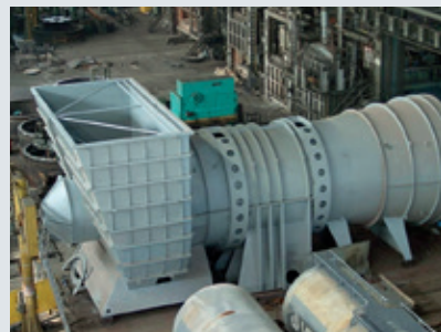
Two stage ID Fan: Trial assembly of casing
