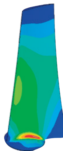
Stress analysis by finite element method
