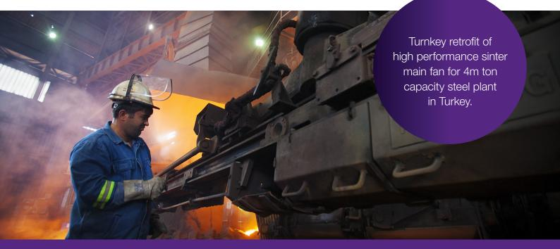
Erdemir Steel needed to bring their sinter plant emission control system into line with European standards while addressing performance issues. Howden's solution was a retrofitted new high performance fan and motor system that eliminates head losses for the electrostatic precipitator while delivering significant annual operational savings.
