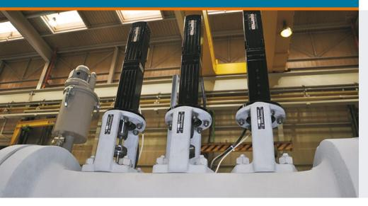
The electromechanical turbine control system enables innovative, reliable and precise control of classic steam turbines.
