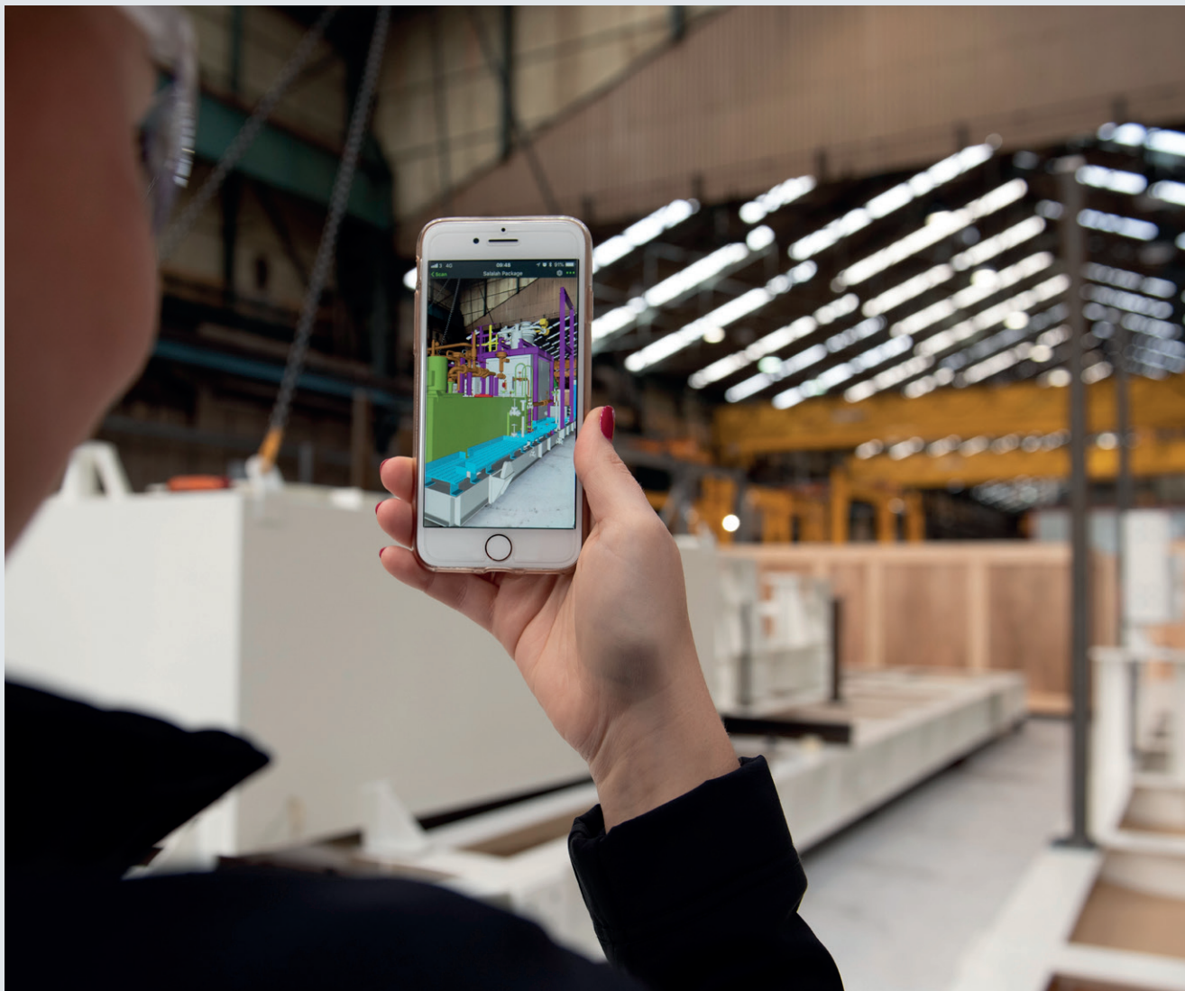
Figure 2: An augmented reality package model sitting directly on top of an empty base frame.
