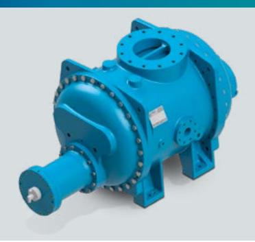
Routine inspection of the compressor is visual inspections and an annual check on thrust bearing wear, however if the unit is fitted with axial displacement probes the need for this annual check is removed, replaced with a review of probe logs.
