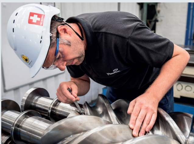
Figure 4: Oil-free compressor rotor clearance check.
