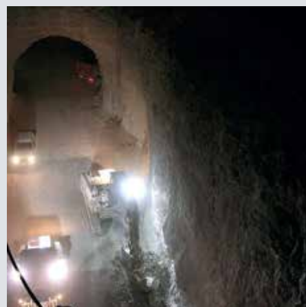
Sector of mine busy with vehicles – Ventsim CONTROL will automatically detect this and adjust airflow accordingly.
