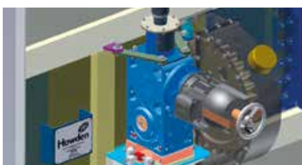
Figure 1: Peripheral drive configuration
