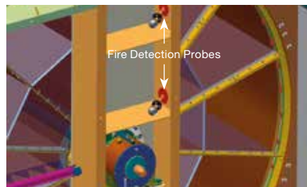
Figure 6: Location of fire detection sensors
