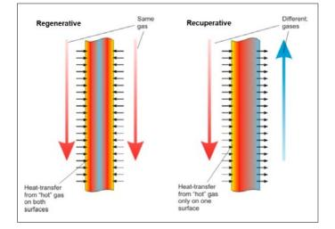
Howden's APH is the regenerative type and carries a number of advantages over recuperative such as the negligible effect on heat transfer caused by fouling as the deposits also absorb and release heat. In addition, efficiency is typically significantly higher within a given footprint (to match the efficiency, a recuperative APH would be much larger).
