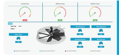
With the collaboration of Twence, Howden has been able to develop a robust condition monitoring system specific for cooling fans installed at ACCs. This system is scalable, cost-effective and able to deliver multiple benefits with respect to maintenance planning and energy savings.
