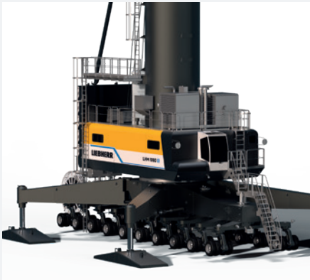
Fans are located in two cabinets on top of the crane motor compartment
