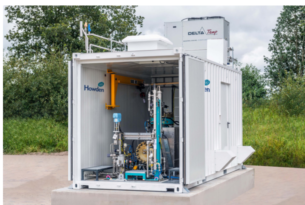
Figure 1. A green hydrogen compression solution with a containerised Howden diaphragm compressor.
