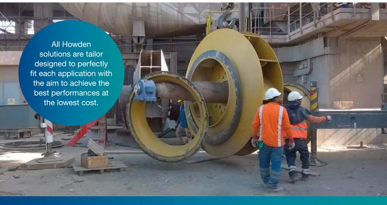
Dust laden is highly present in air and gases that are moved at the cement plant. This dust can have a high concentration in the media that are flowed by cement process fans. As a consequence, depending on the volume and type of dust, fans are subject to increased wear.
