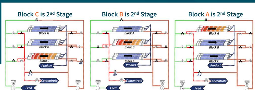
An illustration of the block rotation. In FR-RO, whether it is a 2-stage, or 3-stage system, the pressure vessels are divided into functional rotating blocks. Shown here is a FR-RO adaptation to tapered flow array in a two-stage RO System. The blue pressure vessels are stage one, and the red pressure vessels are stage two.
