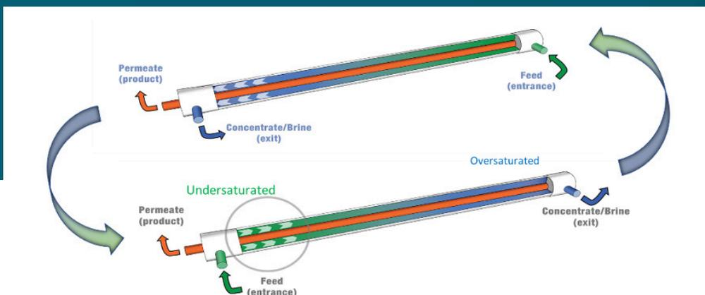
An illustration of the continuous Flow Reversal process in a single pressure vessel. The circled area marks a part of the membrane that, thanks to Flow Reversal, is being continuously flushed by undersaturated water.
