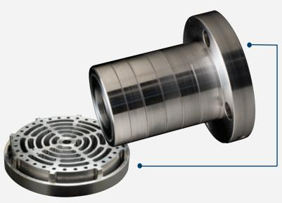
**Piston and Piston Rods** - Services include re-machining of grooves and re-anodizing. Rod reconditioning may consist of machining, grinding, polishing and the application of specialized spray coatings. Finally, all parts are re-assembled with CPI piston and rider rings.
