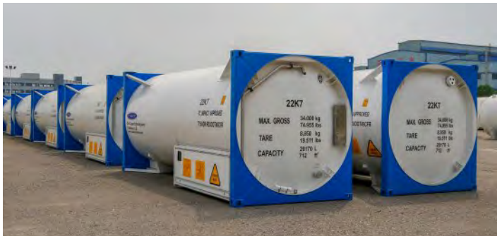
Tank container for refrigerated liquefied gas (UN T75)
