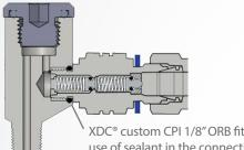
XDC® custom CPI 1/8" ORB fitting eliminates the use of sealant in the connection to the CVP®
