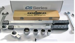
**CS Series** is the sets of Cofimco toolkits specific for installation of each fan model
