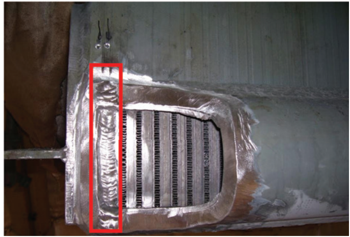
Figure 10. Blocked Layer (encircled in red)
