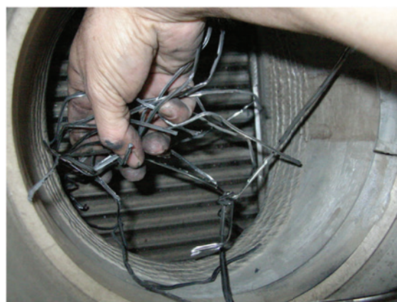
Figure 7. Debris in header/nozzle.
