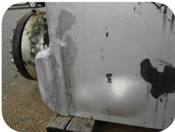
Figure 4. Cap sheet bulge due to ice formation.
