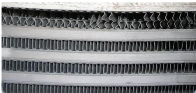
Figure 6. Cracked Distributor Fin
