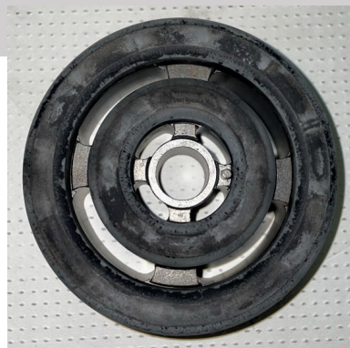
Fig.1 - CPI Hi-FloTM RD valves after 4 years in service
