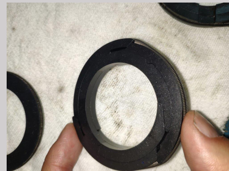
CPI Emissionguard TR 2 packing ring after use
