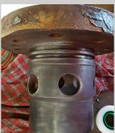
The elements were leaking due to the walls of the valve ports. The components showed a lot of corrosion and superficial pitting. A new valve cover / cage design was required. The addition of new O-rings and gaskets that would improve the seal against the valve port walls and surface of the actuator groove.
