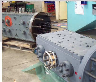
The new cylinder (near) featured thicker and stronger valve port walls, but that required redesigned valves to fit the smaller openings.
