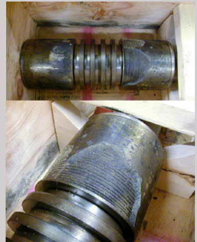
Customer's original single piece piston, showing damage to the sprayed on bronze rider bands
