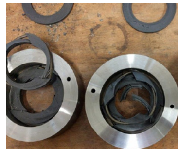
Non-CPI rings after 1,500 hours running life
