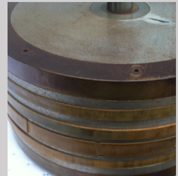
CPI 138 material rings showed no measurable wear at 6 months in service
