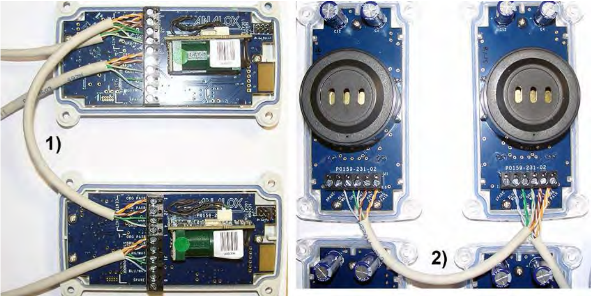
1) Sensors connected via daisy-chain 2) Alarms connected via daisy-chain
