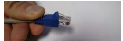
Slide boot back over lock clip
