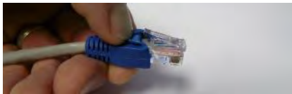
Pull boot back to access lock clip
