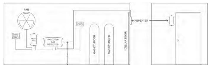
Attach the main unit to the wall 450mm from the floor as close to the valves and manifolds as possible. An 8 metre 8 core cable is pre-wired to the Ax  $50^{TM}$  and has a Remote Alarm Repeater pre-attached. Run the Remote Alarm Repeater cable to the outlet door, safely securing the cable with cable clips.
